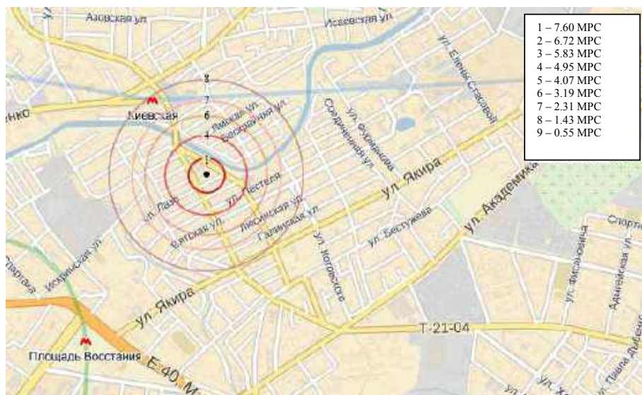
Fig. 3. Calculated dispersion of hydrogen sulfide, released from the water disposal pipeline in the section of the sewer shaft No.51
