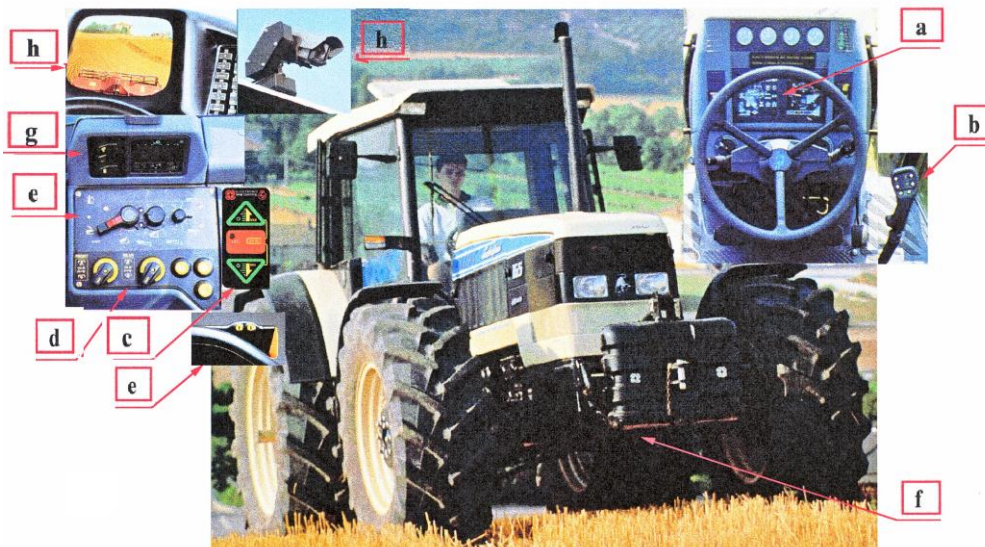
Fig. 2. Lamborghini 165 Racing tractor equipped with board computer (electronic control device): a – control panel showing e.g. witch units are working, gear change, in/of front axis drive, differential mechanism locking, WOM (PTO), work parameters of engine gear box – oil pressure in engine, box, oil temperature, cooling fluid etc. and faults; b – multifunction steering lever – gear change, adjustment of engine rotary velocity, lifting link control; c – engine rotary velocity programmer; d – steering console for front and back WOM (PTO), in/of 4x4 drive, differential mechanism blocking, SBA system; e – lifting link steering panel – up/down, locking, transport, control of up/down speed, adjustment of work parameters (power, position, slippage), alarm, steering keys on wing; f – radar sensor of driving velocity; g – data monitor – shows e.g. tractor velocity, engine and WOM (PTO) rotary velocity, slippage, tool working depth, working width, cultivated area, work period, efficiency etc.; h – camera with monitor for machine watching from tractor back. Source: own elaboration
