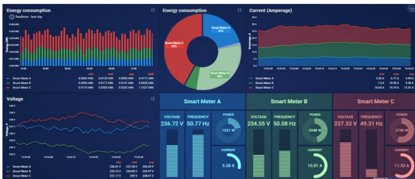
Fig. 29.3 – The ThingBoard Web Application Interface [6]
