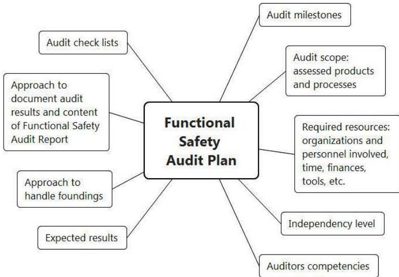
Fig. 25.8 – Structure of Functional Safety Audit Plan
